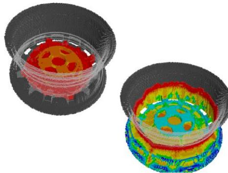
Fig. 8 represents the fluid distribution in improved design 0.42 seconds after Pouring.
