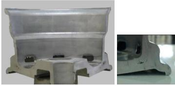
**Fig.3 Shrinkage distribution in real cast part**
