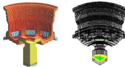
**Fig.7 Shrinkage and thermal distribution in improved design**
